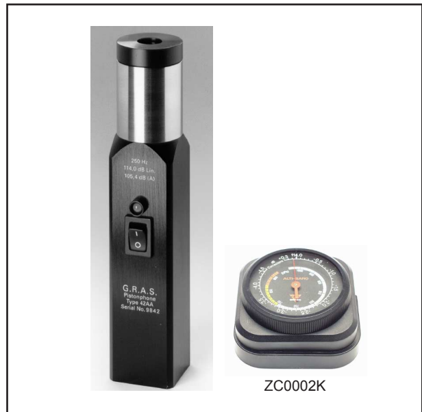
Fig. 1 Pistonphone Type 42AA 114 dB at 250 Hz. Shown with Barometer ZC0002K - for applying corrections for ambient pressure
