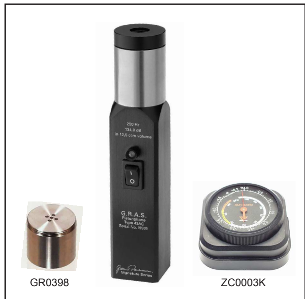
Fig. 1 Pistonphone Type 42AC: 134 dB at 250 Hz. Shown here with Adaptor GR0398 - for hydrophone couplers and Barometer ZC0003K - for applying corrections for ambient pressure
