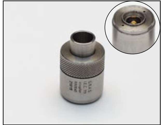
Fig. 1 IEC Ear Simulator Type RA0045 Inset shows built-in Microphone Cartridge Type 40AG
