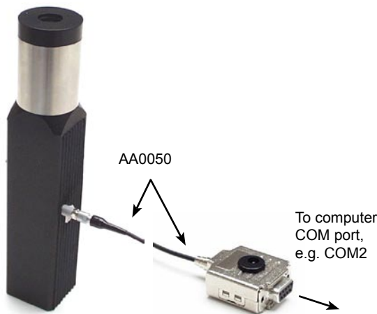
Fig. 2 Pistonphone connection for use with a computer
