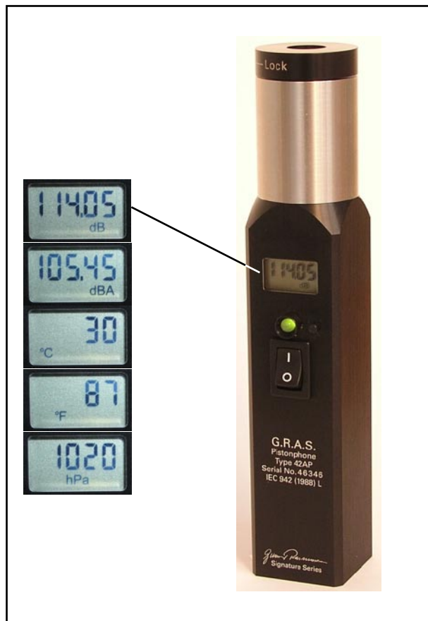
Fig. 1 Pistonphone Type 42AP, 114 dB at 250 Hz shown with an example of each possible display
