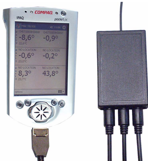
Digital Transducer Adapter 620B/DTA with Handheld and three connected Tilt Sensors 260D/GP
